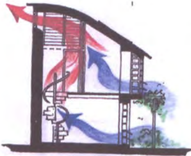
FIGURE 235: The Roman Hut in Christie Walk filters city air through vegetation in a landscape integrated with the building and its neighbours. (Drawn by the author)
