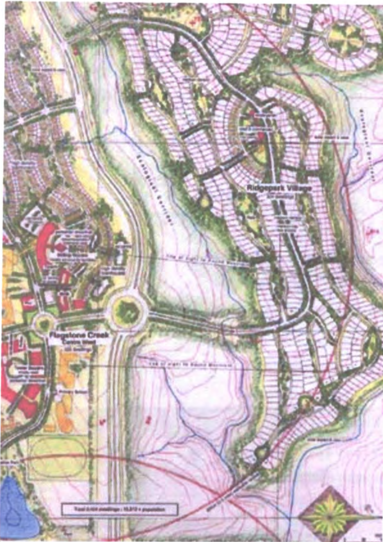
FIGURE 188: Part of a concept plan for a 10,000 population 'new town' for Hall Construction Pty Ltd by the author that was based on ecological corridor planning and walkable city principles. (PFD 1995)
