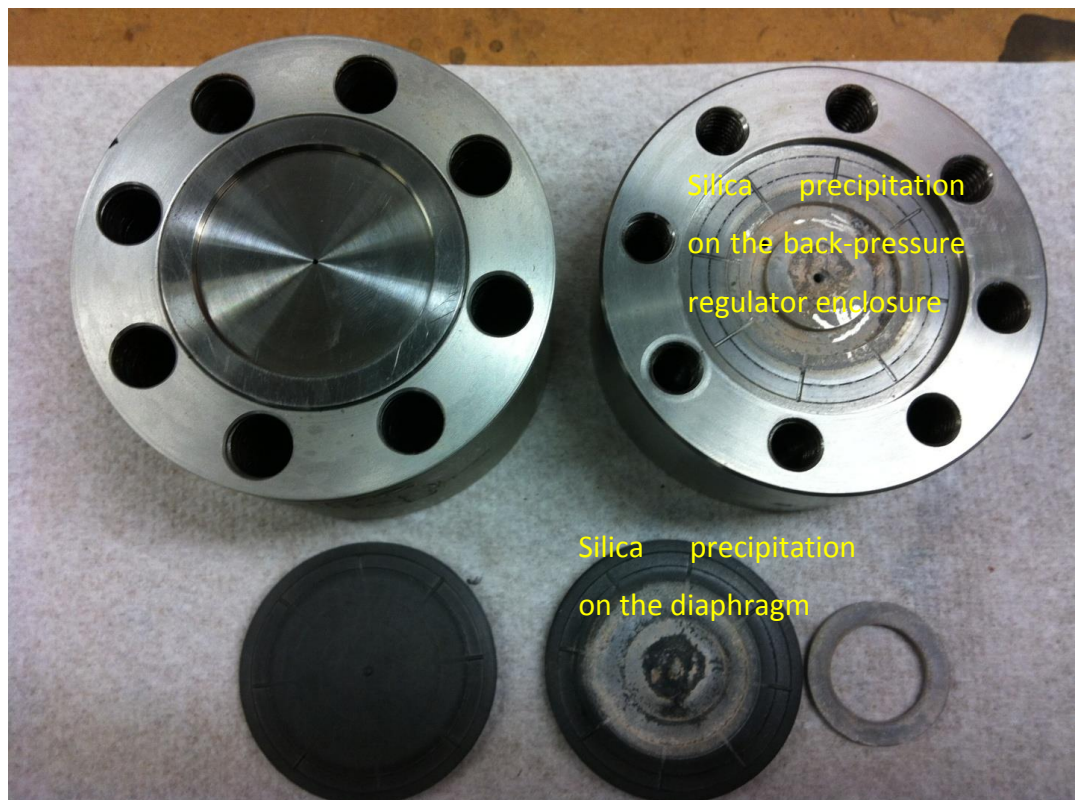
Figure 5.64 Silica precipitation on the diaphragm of a back-pressure regulator
