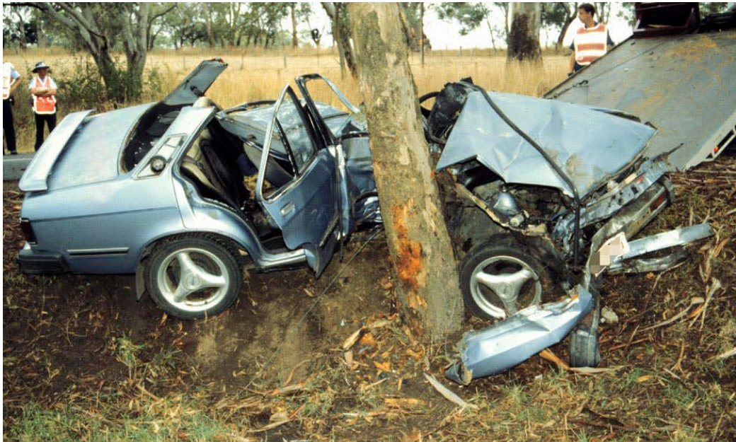
Fig. 6.34: The impacted tree and the damage to the car involved in scenario 6
