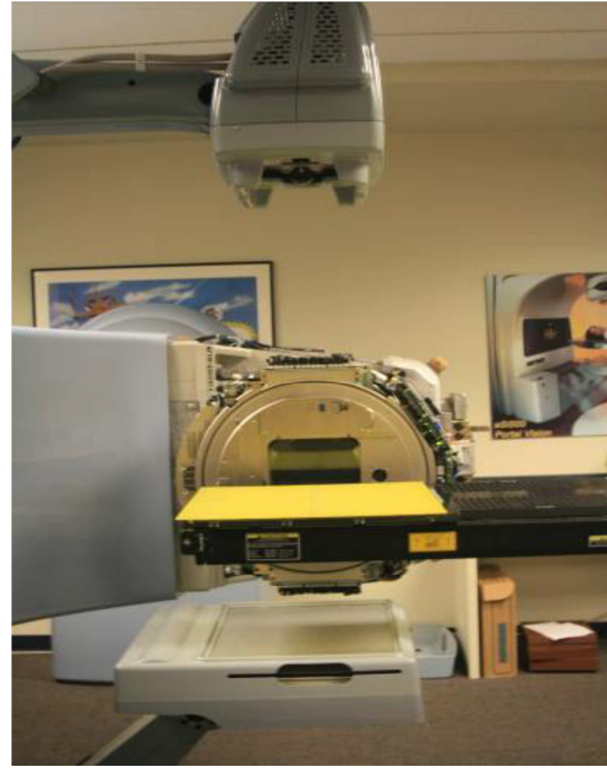
Figure 7.5 (a) Blade calibration plate and (b) setup
