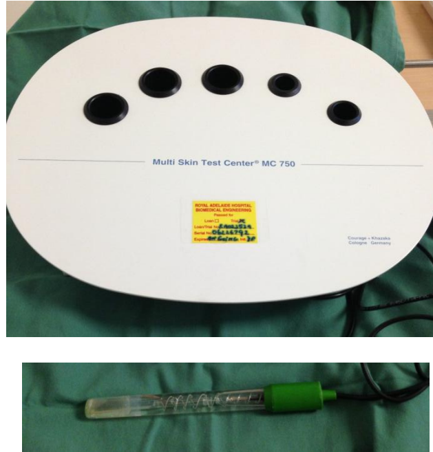
Figure 20 CK® Electronic MC 750 platform and pH probe
