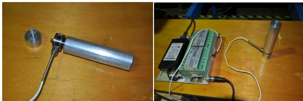
Figures 6.9 (a) and (b): Load cell is screwed onto the aluminium handle
