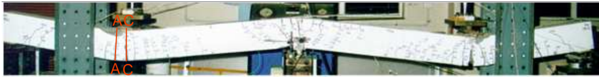
Figure 1: Disturbed regions in RC beam
