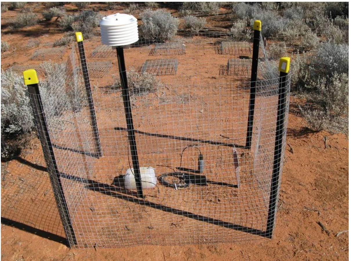
Soil temperature and soil moisture data loggers installed at the study site. Photo: E Steggle
