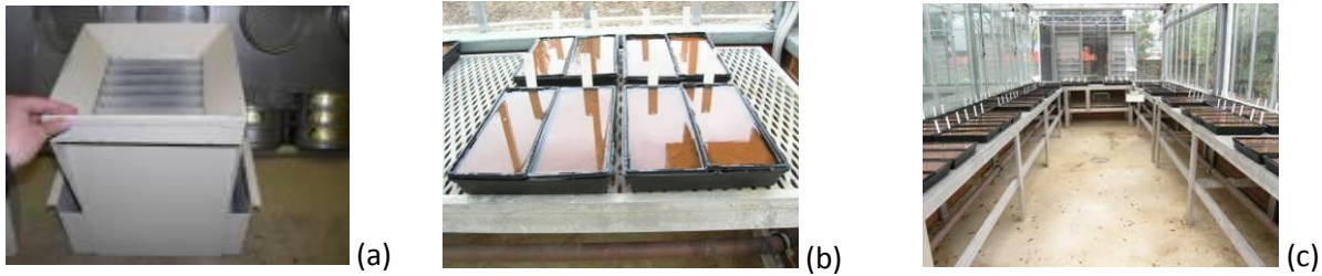
Figure 4-1 Riffle splitter for dividing soil samples into two even sub-samples (a); sub-samples in submerged treatment (b); and layout of seedling trays in the glasshouse (c).
