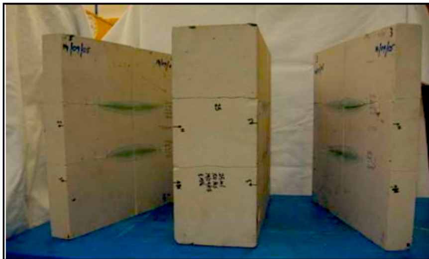
Figure 19. Fracture growth through discontinuities
