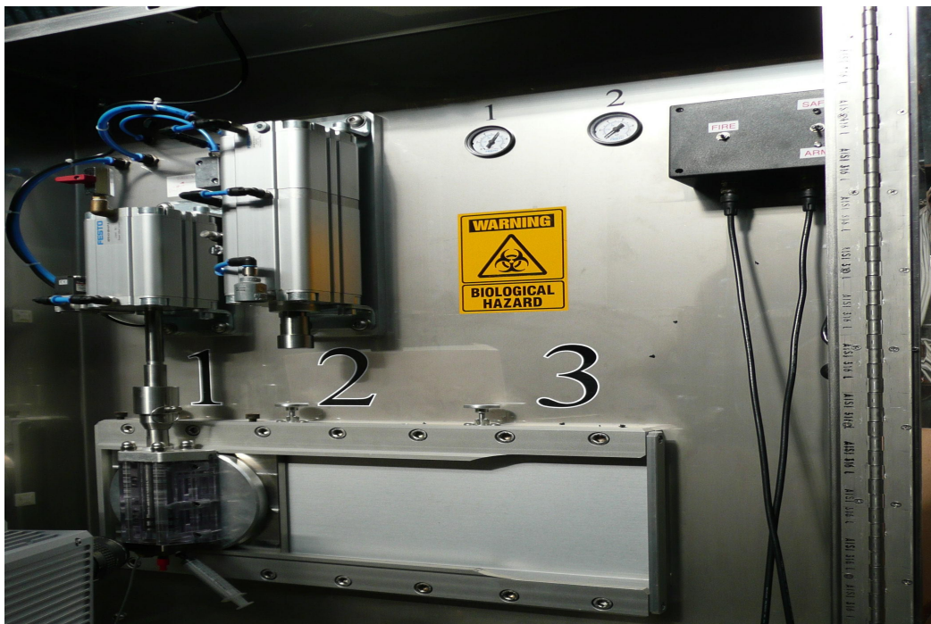
Figure 6.3 (b) Front view showing the extensive high pressure lines (blue), the primary functional mechanism of the apparatus.
