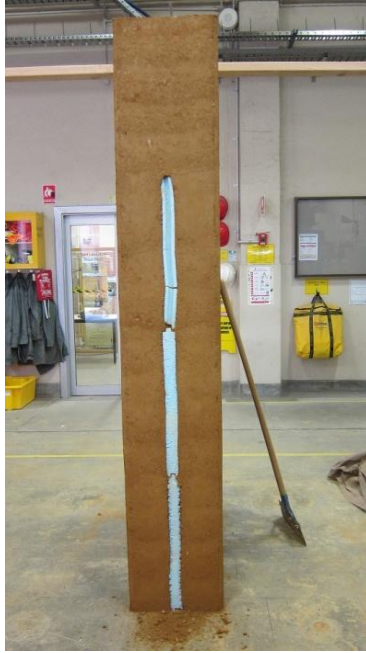
Figure 2.3 Insulated cavity rammed earth wall
