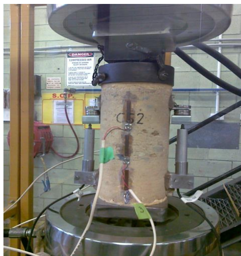
Figure 5 Test setup for compression test of molded cylindrical specimens
