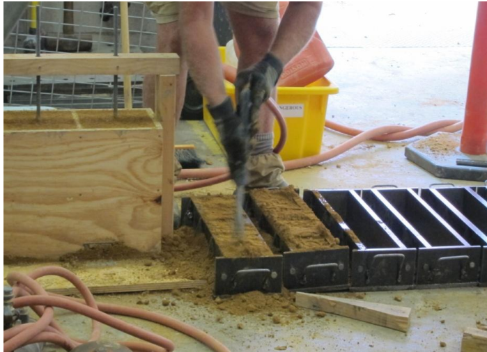
Figure 2 Construction of material test specimens
