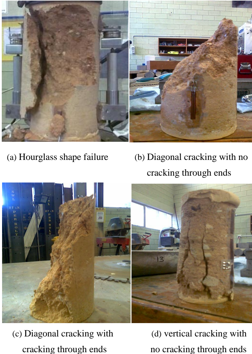
Figure 6 Typical failure patterns of cylindrical specimens
