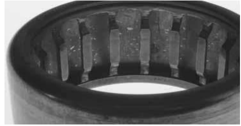
(b) Bruising due to particle contamination of lubricant.
