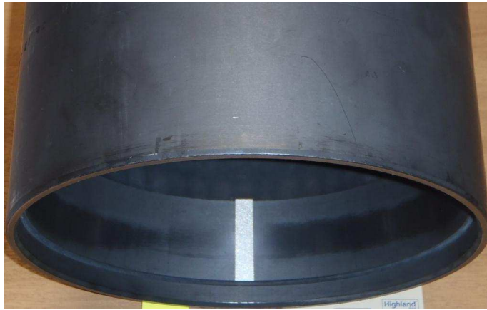
Figure 5.1: A photo of the line spall of circumferential length L_d = 10 mm and depth H_d = 0.2 mm machined on the outer raceway of the bearing using electric spark erosion.
