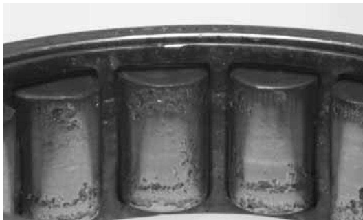
(a) A few point spalls on the rolling elements.
