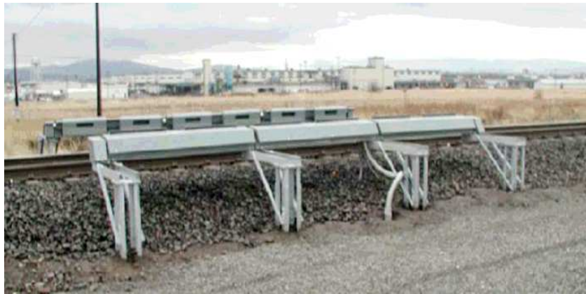
Figure 1.2: A photo of the TADS ® system [12] showing the wayside cabinets (courtesy: TTCI ® [13]).
