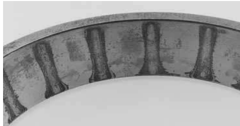
(c) Corrosion due to etching.
