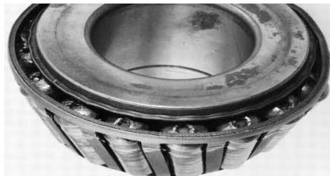
(e) Race deformation due to excessive heat generation.
