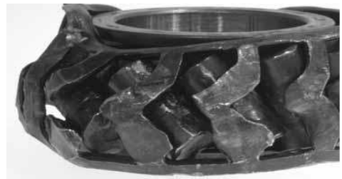
(f) Complete bearing lockup due to inadequate lubrication.
