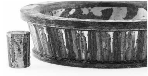
(d) Severe corrosion due to etching.
