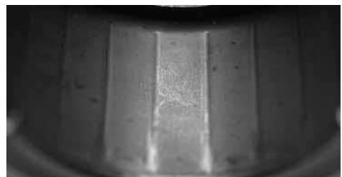
(h) True brinelling due to shock loading.
