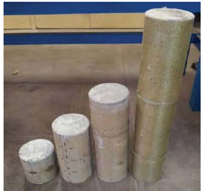
Figure 7: CFFT specimens prepared with H/D ratios of 1, 2, 3 and 5.
