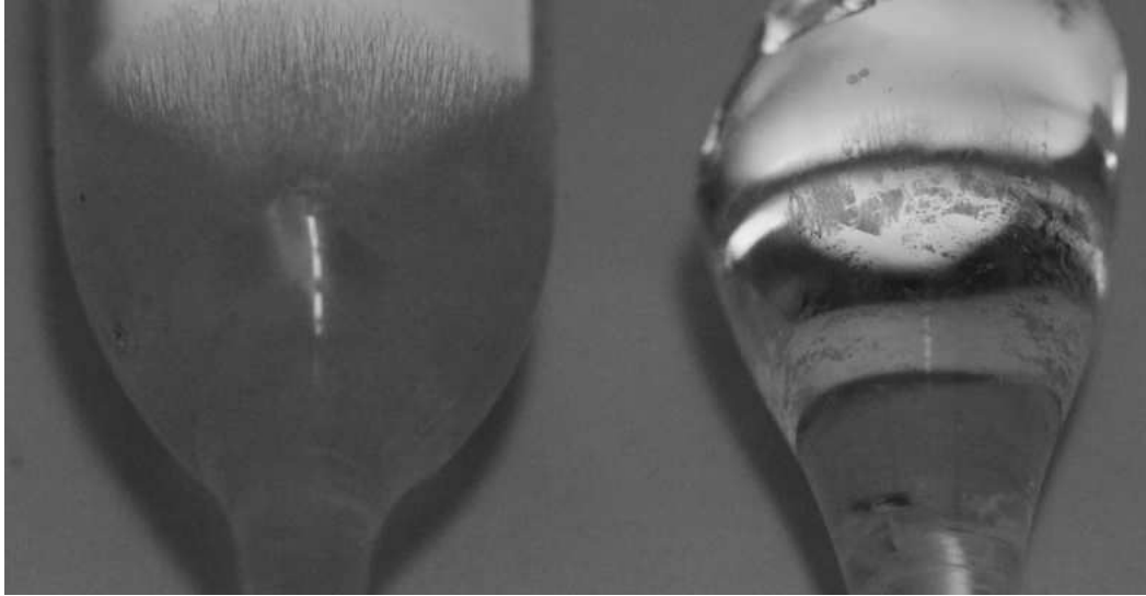
Figure 4.10: Comparison of neckdown region between (a) unpolished and (b) polished preforms. All other fabrication conditions were constant.
