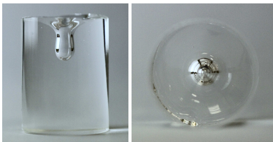
Figure 4.15: \text{Tb}^{3+} -doped FP glass billet, polished in preparation for extrusion. \text{Tb}^{3+} -concentration is 7200 ppmwt, billet mass is 102.6 g.
