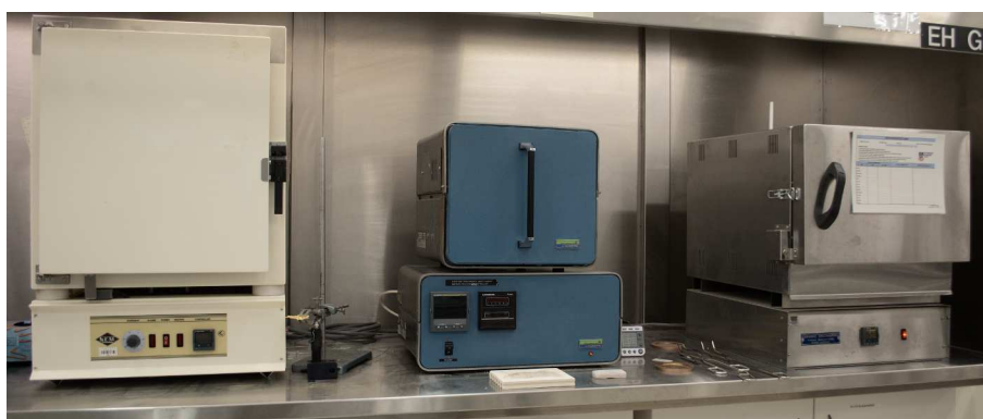
Figure B.2: Glass melting facilities. Top: nitrogen atmosphere glovebox for batching and melting of fluoride glasses. Bottom: open air melting and annealing furnaces.
