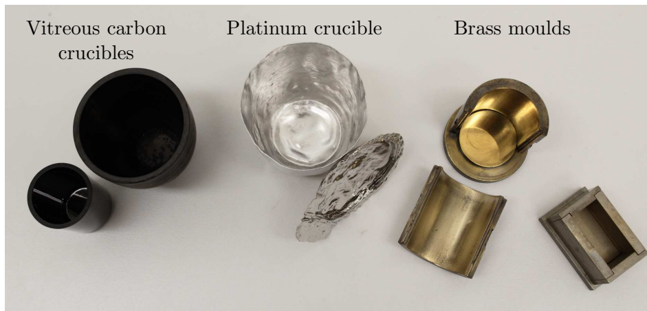
Figure B.3: Crucibles and glass moulds used for remelting and doping of FP glasses. Vitreous carbon crucibles are used for reducing environment melts; the platinum crucible is used for open air, oxidising environment melts. Brass moulds are polished before use.
