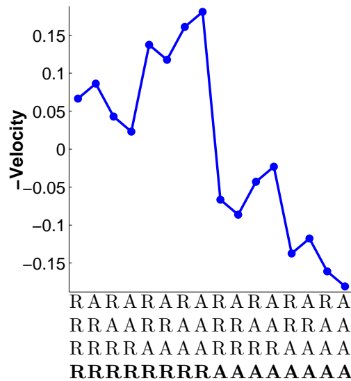
FIGURE 4.9: Results of an oscillator set to resonate with alternations (ALT). The curve shows velocity measurements taken just before the last pulse and take into account whether the last stimulus was expected or not (see main text). The natural frequency of the oscillator is set to match the alternation frequency so \omega_0 = f_{REP} = 0.5 Hz; damping was set at \gamma = 1.5 for this example. Note how results are almost perfectly symmetrical with those of an oscillator tuned to f_{REP} shown in Figure 4.8, except for a slightly greater amplitude of ALT compared to REP (see main text).
