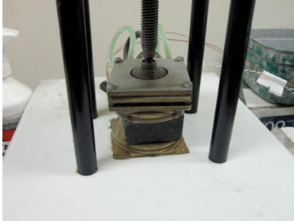
Figure A4.2 – The vertical section of the PEDB apparatus, showing the sample in place between the two brass plates.
