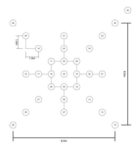
Figure 1. Layout of the cone penetration soundings
