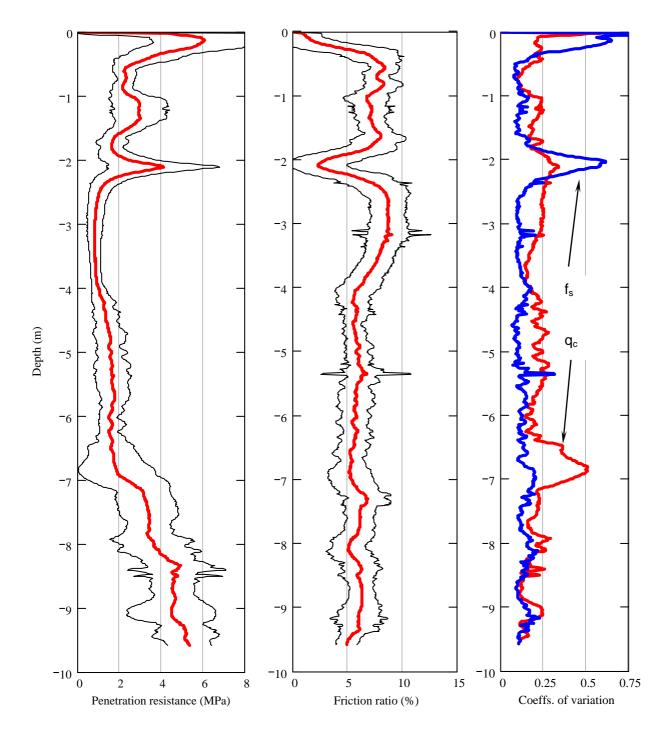
Figure 2. CPT data averaged at each depth. Left:  $q_c$ , middle:  $f_s$ , right: coefficients of variation of  $q_c$  and  $f_s$ .
