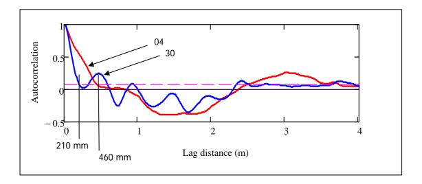
Figure 5. Autocorrelation functions for CPT 04 and CPT 30 showing the scale of variability in the vertical direction of 460 and 210 mm respectively.
