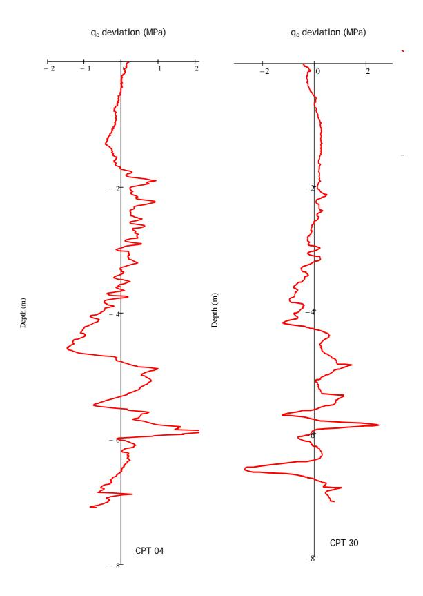
Figure 4. De-trended plots for  $q_c$  deviations for CPT 04 and CPT 30
