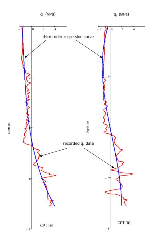
Figure 3. Data for CPT 04 and CPT 30: recorded  $q_c$  data minus the mean value at each level ( $q_c$  deviations) along with the third order polynomial regression curve.
