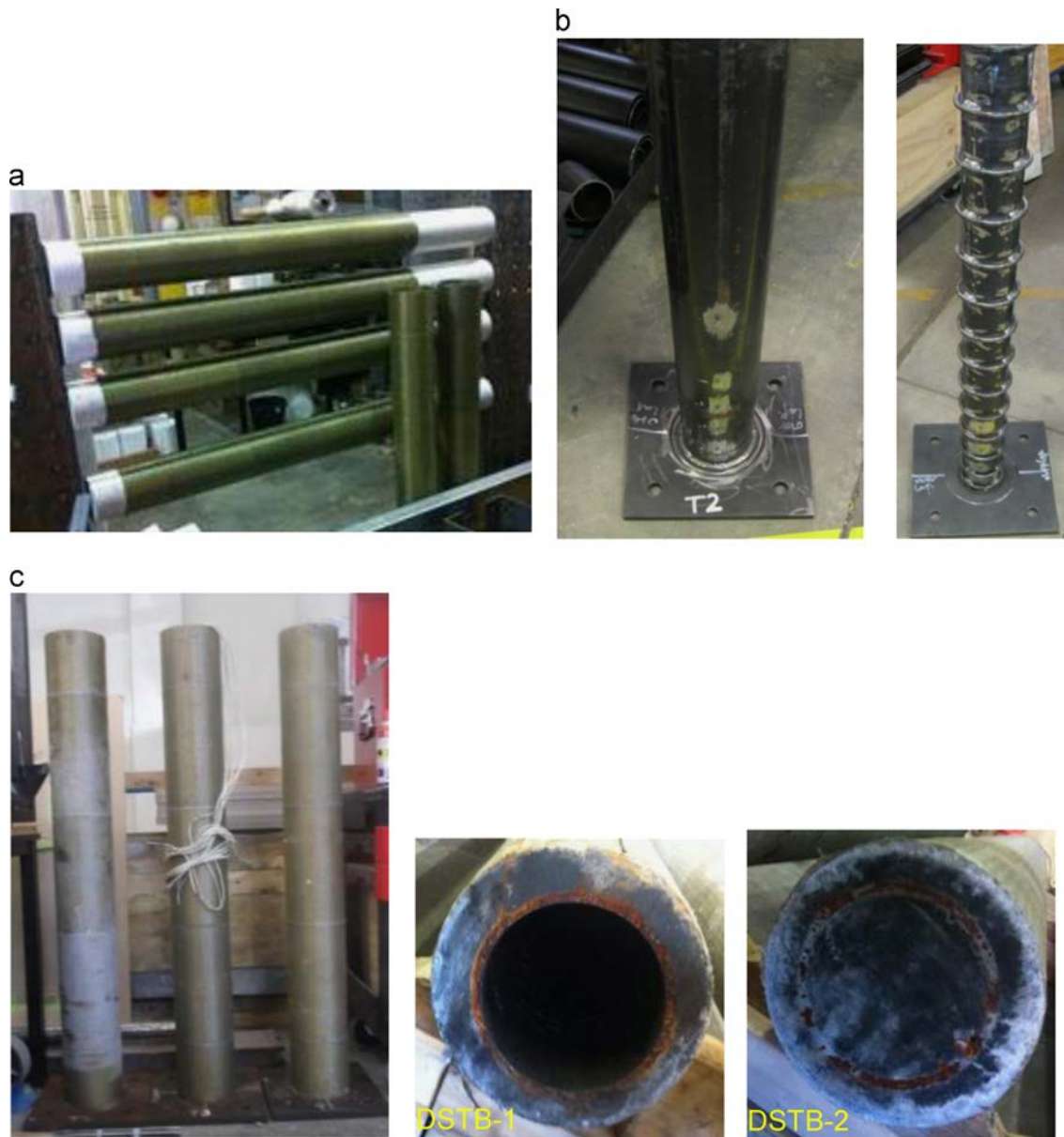
Fig. 2. Manufacturing process: (a) Steel tubes; (b) Manufacturing of FRP tubes; (c) Specimens after concrete pouring
