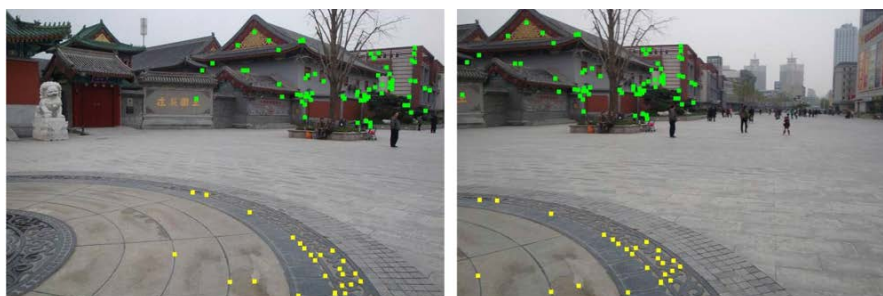
(a) The images to stitch and the clustered ground and distant plane SIFT matches (in yellow and green colour, respectively).
