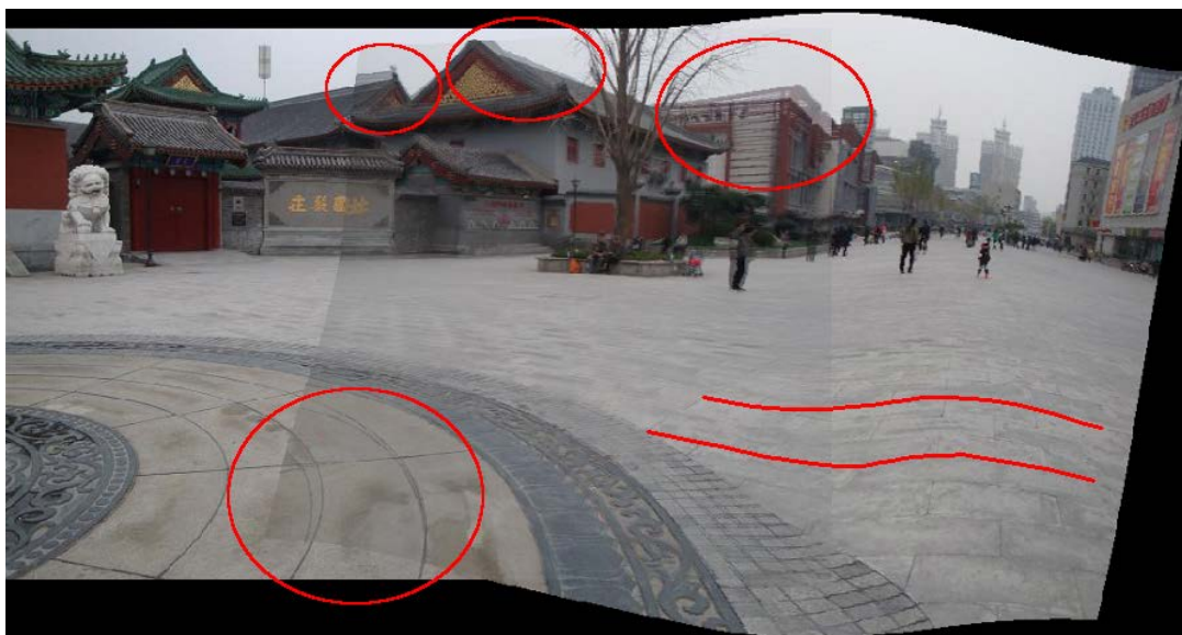
Figure 4.5: Image stitching results obtained with as-affine-as-possible warps generated with MLS. Note the distortion of the alignments in the areas where the images do not overlap. The two red strokes drawn on top of the images illustrate the deformations of the warp. These strokes follow the lines of the tiles of the floor. Besides the image distortions, visible alignment mistakes remain (circled in red). This is probably a consequence of the implicit bias which constrains the flexibility of the alignments when there is few data to guide the warps. The images are taken with a camera undergoing rotation and translation. The size of the images is 730 \times 487 pixels. The number of inliers after RANSAC is 415. Similar to Fig. 4.2, the domain of image I was partitioned into 100 \times 100 cells.
