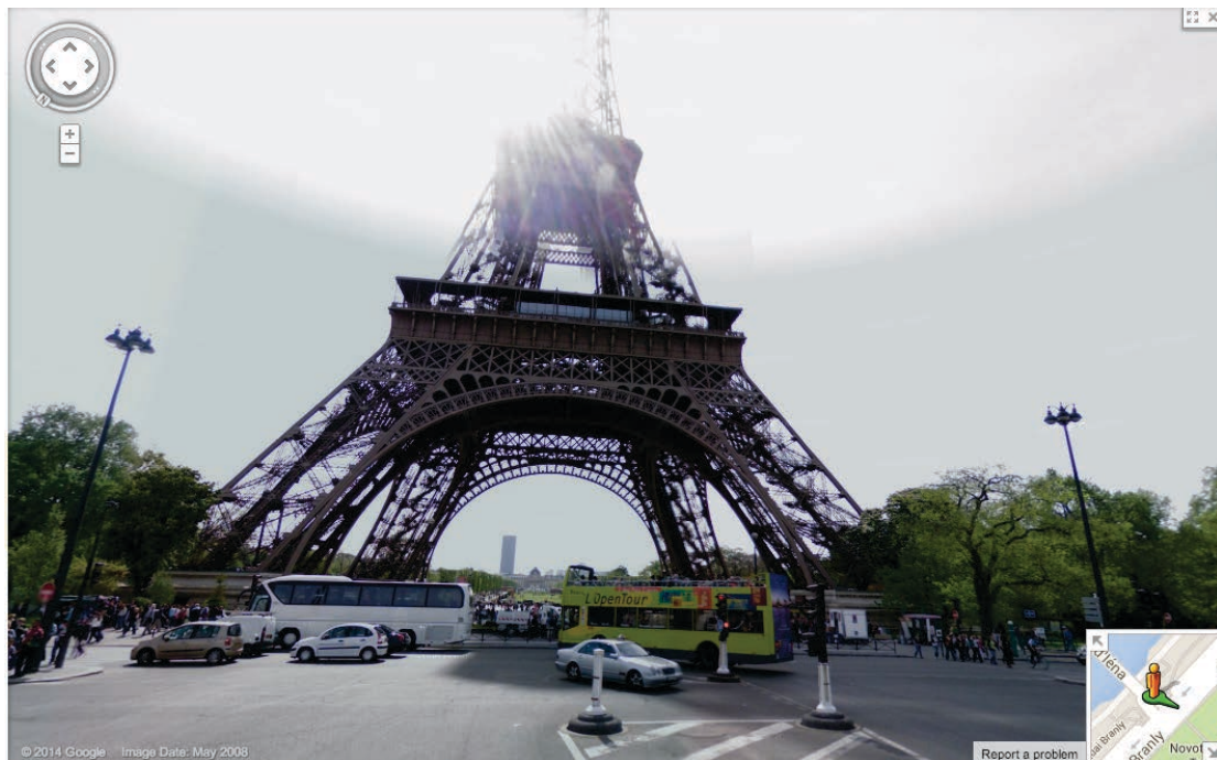
Figure 1.2: One of the panoramas generated by Google’s street views. The panoramas are generated by stitching frames of videos taken with specially adapted vehicles like cars, tricycles, boats or snowmobiles.
