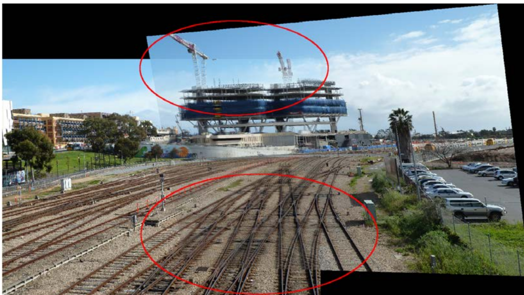
(c) Image alignment results obtained by means of a basic homography warp. As can be seen in this image, due to the images deviating from the idealised conditions of the homography warp, several alignment mistakes (circled in red) can be observed.
