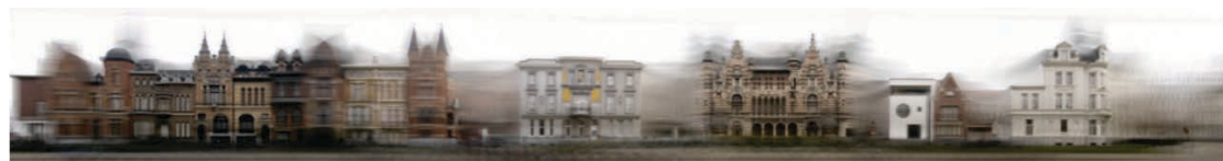
(b) A panorama generated by projecting a set of images into a user defined reference plane. This panorama is composited with simple image average blending.
