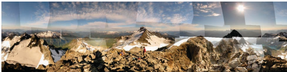
Figure 3.4: An example of a panorama generated by means of Brown and Lowe's Bundle Adjustment method [12]. The panorama is composited with simple pixel average blending. This panorama was taken from [12].
